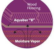
Aquabar "B" helps slow moisture vapor originating below the wood floor system.
